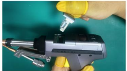
② Remove the protective lens holder
