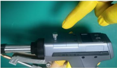
① Unscrew the protective lens screw
